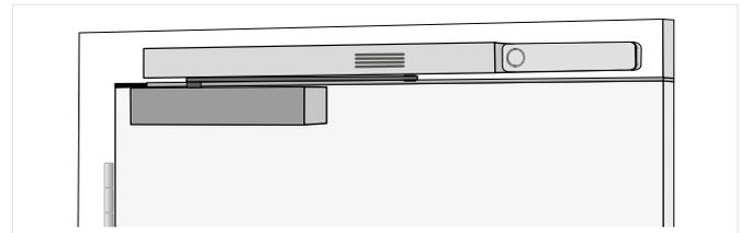
Abb. 4: Montageposition Konsole FM 155 F
