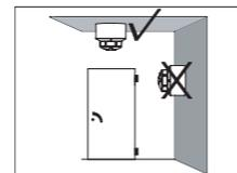
The Smoke Switch ORS 142 must be mounted as shown in the illustration. It must only be mounted on a horizontal surface with a minimum distance of 0.5 m to any installations.
